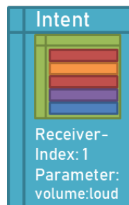
Figure 3.3 – The Intent containing the task object, the receiver index and a parameter "volume".
